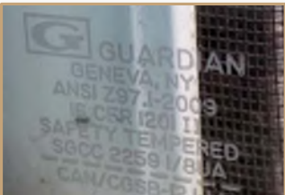
Example of etched label on the corner of tempered glass
